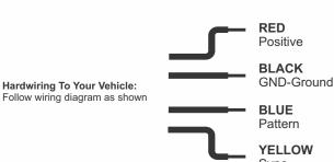
**1. Changing Patterns:** Patterns can be changed by momentarily connecting the blue wire to the ground of your vehicle's battery.
