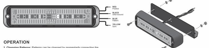
**1. Changing Patterns:** Patterns can be changed by momentarily connecting the blue wire to the ground of your vehicle's battery.
